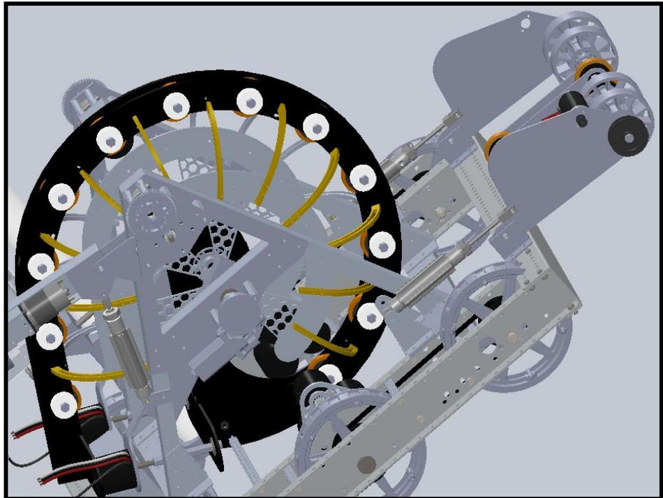
and some support bars so it fit together, even with the movement of our manipulators. We then changed the piston mount to the spinner module. It is now two separate parts as a sub assembly. The engineers from the review also encouraged us to make the intake cad more sturdy, leading us to go back and strengthen it.
